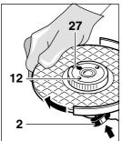
grinder Lock the spindle with the spindle lock button 2. Tighten the guicknut by clamping forcefully turning the grinding disc in the clockwise direction.
