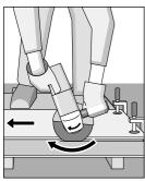
The direction in which the cutting is performed is important.
