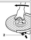
A properly tightened undamaged, guickclamping nut can be loosened by hand turning the knurled ring in anticlockwise direction.
