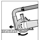
The vacuum cleaner must be approved for the extraction of masonry dust.
